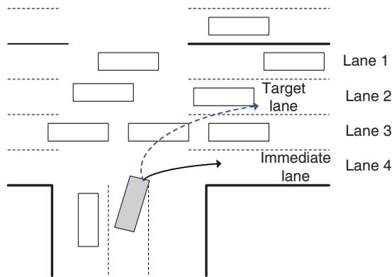
Figure 9. Example of a situation when the target lane is blocked.
